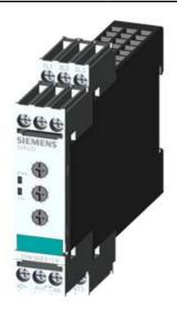
SOFT STARTER WIDTH 22.5 MM 3A, 1.1KW/400 V, 40 DEGR.C 200-400V / UC 24-230V SCREW CONNECTION
